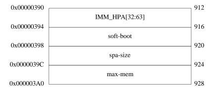
The IMM\_HPA word is the HPA of the Initial Memory Module. IMM\_HPA[32:63] contains the least significant 32 bits of the HPA of the Initial Memory Module. If IMM\_HPA[0:31] is zero, then IMM\_HPA[32:63] must be F extended to form a 64 bit address. If IMM\_HPA[0:31] is not zero then it will be concatenated in the high order 32 bits to form a 64 bit address.
