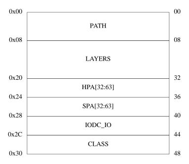
The Console/Display, Boot Device, and Keyboard Extensions are 8 bytes, the first 4 bytes (offset 0) contain HPA[0:31] for the module, and the next 4 bytes contain SPA[0:31] for the module.
